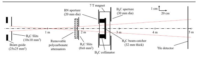
FIG. 2. Schematic of the experiment at beamline 4A at SNS. Description in the text.
